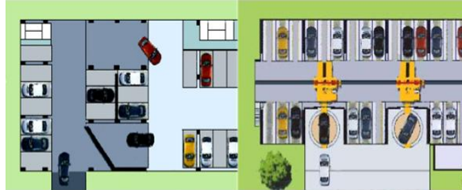
Fig. 1 Traditional Parking v/s Automated Parking
