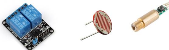
Fig. 5 LDR Circuit and LASER Module
